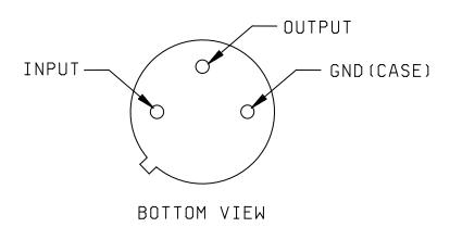
FIGURE 2. <u>Terminal connections</u>.
